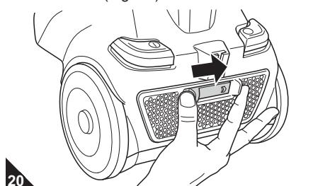
3. Remove the exhaust filter.
