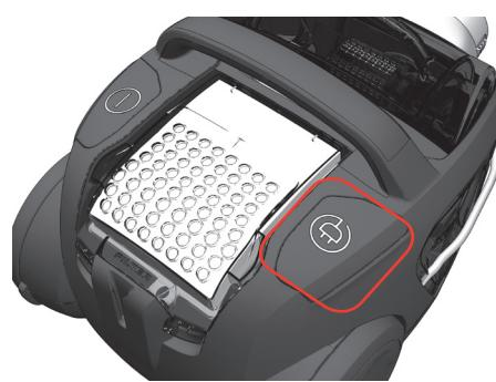
**After vacuuming rewind the power cord by pushing the REWIND button.**
