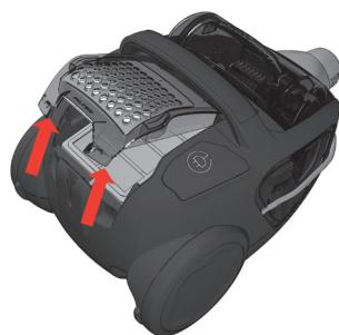
Open the filter lid by pulling the back edge backwards and upwards.
