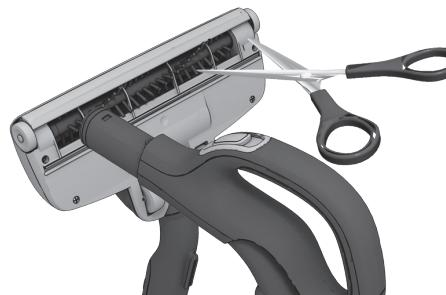
Disconnect the nozzle from the vacuum cleaner tube and remove entangled threads, etc. by snipping them off with scissors. Use the hose handle to clean the nozzle.
