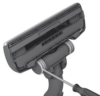
If the wheels are stuck, clean them by removing the wheel cap (only at the AeroPro nozzle) with a small screwdriver.
