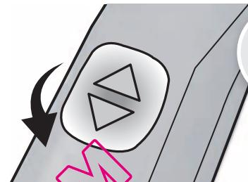
**3. Adjust the power level by pushing the lower part of the on/off button:**
