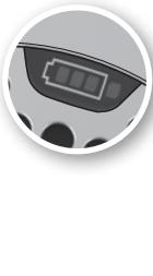
**2. Ergorapido Plus:** The battery capacity display lights will come on one after another as the machine is charging after being positioned correctly in the charging station.
