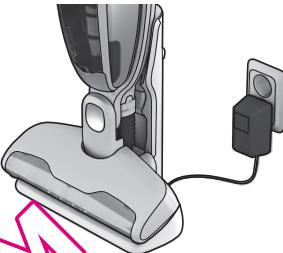
**3. When fully discharged,** approximately 16 hours' charging is required to regain full battery capacity (4 hours for Ergorapido Plus). Leave Ergorapido on charge when not used to maintain battery performance.
