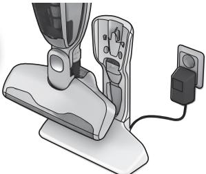
**1. Ergorapido:** The indicator light will come on once the Ergorapido is positioned correctly in the charging station. When fully charged, the LED will be on for a few seconds per minute.
