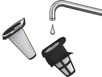
4b.Separate both filters. Dust container and filters can be shaken clean or rinsed in warm water (never in dishwasher). All parts must be dry before reassembled in reverse order.
