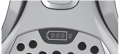
**4. When fully charged** the LED's\* will turn off and go into standby mode = much lower power consumption, indicated with one blink per minute.
